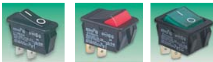
273-211 273-247 521-930 Single pole : Bezel=33.4x14.0, Depth=16.2, Panel cut-out=30 x 11, Tab=6.3 x 0.8 Double pole : Bezel=33.4 x 25.0, Depth=16.2, Panel cut-out=30 x 22.1, Tab=6.3 x 0.8
